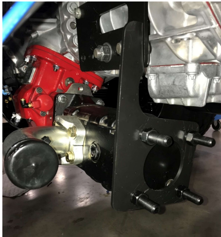
Figure 43: Actual Bottom PTO support bracket, pic 2
